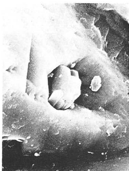
Fig. 8. Crystalline inhomogeneity (sphalerite?) in pyrite, SEM, \times 9000 (1385–1397.5 m).
