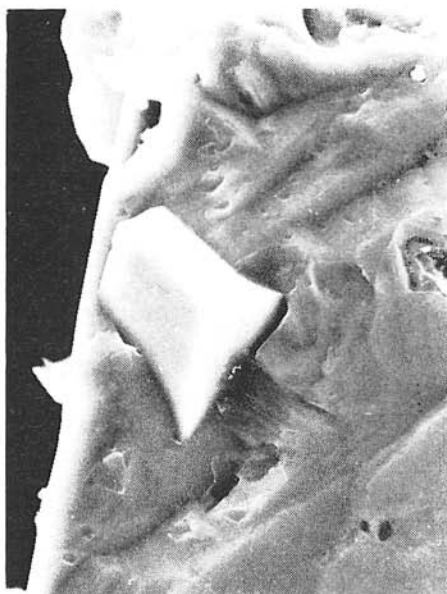
Fig. 7. Cubic (octahedral) electrum in pyrite from the lower part of borehole, \times 2250 (1385–1397.5 m).
