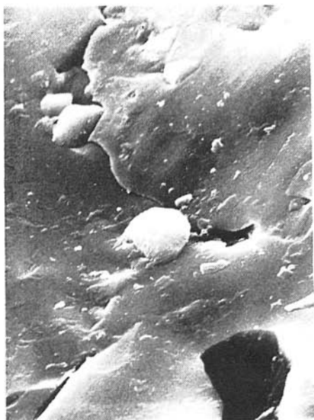
Fig. 5. Globularly rounded, colloform enclosures of electrum in pyrites occurring on the borders of block structure, SEM, \times 6000 (1004–1017 m).
