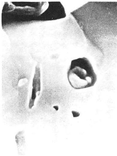
Fig. 6. Globular forms of electrum with marked microtexture (by striation), SEM, \times 30\,000 (805–828 m).
